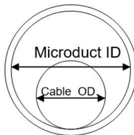
**Figure 1 – Cable and microduct dimensions for use in diameter and area ratio calculations.**
