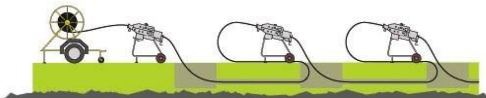
Figure 3 – Cascaded blowing machines. (Note: For clarity, the air compressors are not shown in Figure 3.)
